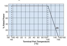
For resistors operated at an ambient temperature of 105°C or above, a power rating shall be derated in accordance with the above derating curve.
