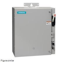
Pump control panel, Size 2, Three phase full voltage, Solid-state overload relay, OLR amp range 13-52A, 240V 50Hz / 277V 60Hz coil, Standard type contactor, 50A circuit breaker, HOA Sel Sw. </>&<)> Start P.B., Enclosure NEMA type 3/3R, Weather proof outdoor use
