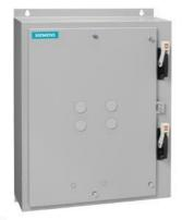
Duplex starter w/ alternator, Size 3 1/2, Three phase full voltage, Solid-state overload relay, OLR amp range 50-200A, 110V 50Hz / 120V 60Hz coil, Combination type, Two 125A circuit breakers, Encl NEMA type 4X 304 S-Steel, Water/dust tight noncorrosive
