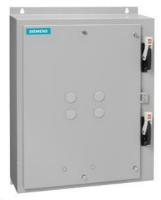
Duplex starter w/o alternator Size 3 Three phase full voltage Solid-state overload relay OLR amp range 25-100A 208VAC 60Hz Coil Combination type Two 100A disconnect switches Enclosure NEMA type 1 Indoor general purpose use
