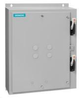
Duplex starter w/o alternator Size 1 Three phase full voltage Solid-state overload relay OLR amp range 0.25-1A 208VAC 60Hz Coil Combination type Two 30A disconnect switches Enclosure NEMA type 1 Indoor general purpose use
