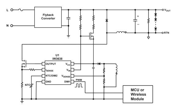
Figure 3.1 : iW3638 Typical Application Circuit (Wireless Dimming with NTC Derating Using Depletion-mode FET as Active Start-up Device)
