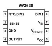
Figure 4.1: 8-Lead SOIC-8 Package
