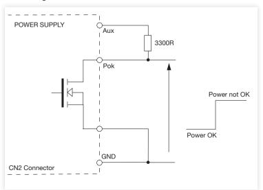
Open drain signal, low when PSU turns on. Maximum sink current: 20mA Maximum drain voltage: 40V
