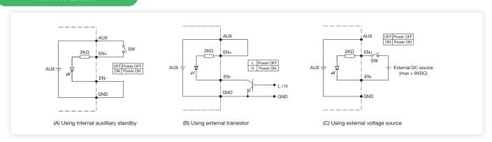
\*GND shown in above diagram is referring to the GND of CN5, not the grounding from output power (NEG (-))
