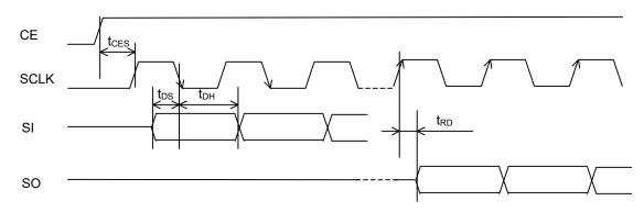
Conversely, when the SCLK pin is held high in the low to high transition of the CE pin, the models will select the timing with which the SO pin output is synchronized with the falling edge of the SCLK pin input, and the SI pin input is synchronized with the rising edge of the SCLK pin input, as illustrated in the timing chart below.
