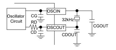
\*1) The CGOUT or/and CDOUT should have a capacitance ranging from 0 to 6 pF.
