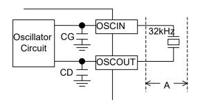
Typical externally-equipped element X'tal : 32.768kHz (R1=50kΩ typ) (CL=6pF to 9pF) Standard values of internal elements CG,CD 10pF typ
