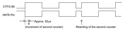
In the pulse mode, the increment of the second counter is delayed by approximately 92  $\mu$ s from the falling edge of clock pulses. Consequently, time readings immediately after the falling edge of clock pulses may appear to lag behind the time counts of the real-time clocks by approximately 1 second. Rewriting the second counter will reset the other time counters of less than 1 second, driving the /INTR pin low.
