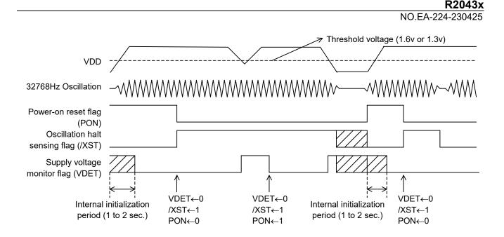
When the PON bit is set to 1 in the control register 2, the DEV, F6 to F0, WALE, DALE, /12·24, /CLEN2, TEST, CT2, CT1, CT0, VDSL, VDET, /CLEN1, CTFG, WAFG, and DAFG bits are reset to 0 in the oscillation adjustment register, the control register 1, and the control register 2. The PON bit is also set to 1 at power-on from 0v.
