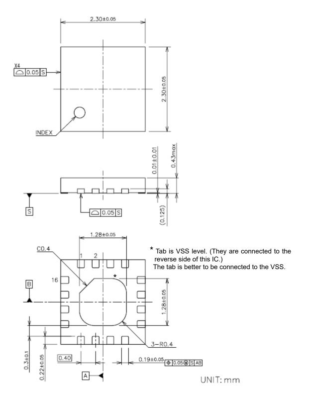
※ The side of the all terminals have no plating treatment. Therefore, it may not be able to form solder fillet on the side of the terminals. \* R2043L (QFN023023-16) is the discontinued product as of May, 2023. \* R2043K (FFP12) is the discontinued product as of July, 2016.
