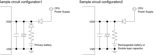
\*Set bypass capacitors as close as possible to the IC, use a capacitor for high frequency and another capacitor for low frequency in parallel.
