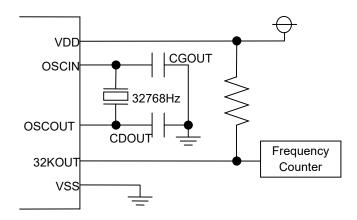
X'tal : 32.768kHz (R1=50kΩ typ) (CL=6pF to 9pF) Topt : 25°C Output pins : Open
