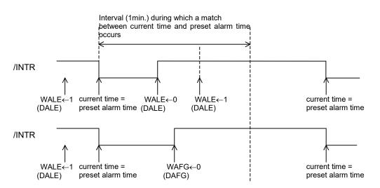
After setting WALE(DALW) to 0, Alarm registers is set to current time, and WALE(DALE) is set to 1, /INTR will be not driven to "L" immediately, /INTR will be driven to "L" at next alarm setting time.
