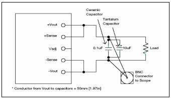
Output ripple and noise test setup
