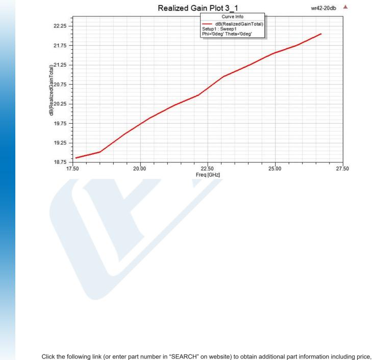
inventory and certifications: WR-42 Standard Gain Horn with 20 dBi gain, 2.92mm Female connector PEWAN042-20KF
