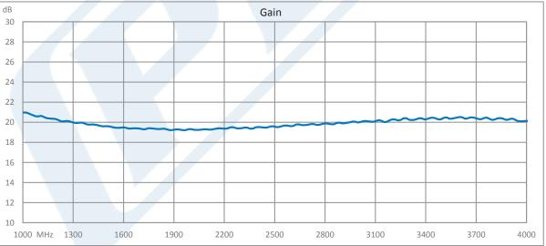
Click the following link (or enter part number in "SEARCH" on website) to obtain additional part information including price, inventory and certifications: 41 dBm IP3, 0.8 dB NF, 22 dBm Psat, 1 GHz to 4 GHz, Low Noise Amplifier, 20 dB Gain, SMA PE15A1070
