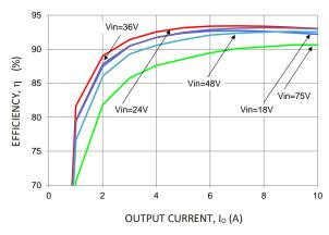
Figure 1. Converter Efficiency versus Output Current.
