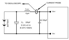
NOTE: Measure input reflected ripple current with a simulated source inductance ( $L_{TST}$ ) of 12µH. Capacitor C<sub>S</sub> offsets possible battery impedance. Measure current as shown above.
