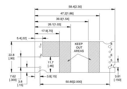
TH Recommended Pad Layout (Component Side View)
