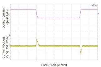
Figure 3. Transient Response to 0.1A/µS Dynamic Load Change from 50% to 75% to 50% of full load, Vin=24V.
