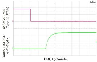
Figure 5. Typical Start-up Using Remote On/Off, negative logic version shown ( $V_{IN} = 24V$ ,  $I_0 = I_{0,max}$ ).
