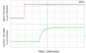
Figure 6. Typical Start-up Using Input Voltage ( $V_{IN}$  = 24V,  $I_0$  =  $I_{O,max}$ ).
