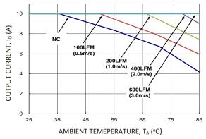
Figure 18. Output Current Derating for the Open Frame Module; Airflow in the Transverse Direction from  $V_{out}(-)$  to  $V_{out}(+)$ ;  $V_{IN}$  =24V,  $V_0$ =12V.
