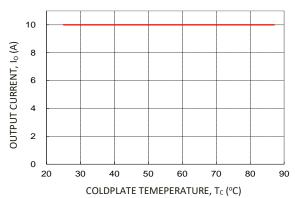
Figure 22. Derated Output Current versus Cold Wall Temperature with local ambient temperature around module at 85C;  $V_{\rm IN}$  =24V or 48V.
