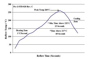
Figure 26. Recommended linear reflow profile using Sn/Ag/Cu solder.
