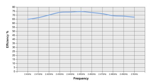
All data measured on SRFW082-100 in a loaded condition adhered to a plastic carrier in free space.
