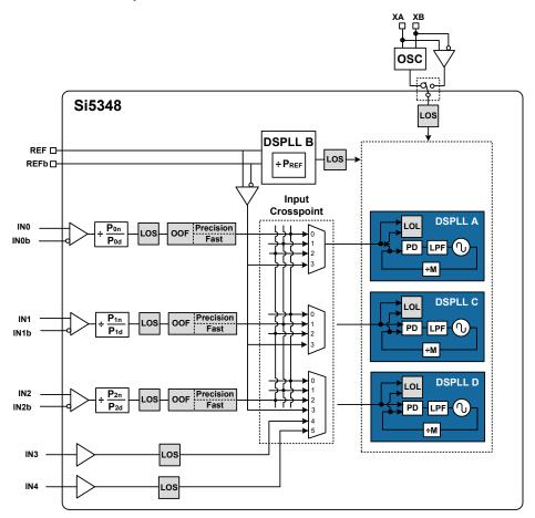
Figure 4.10. Si5348 Fault Monitors
