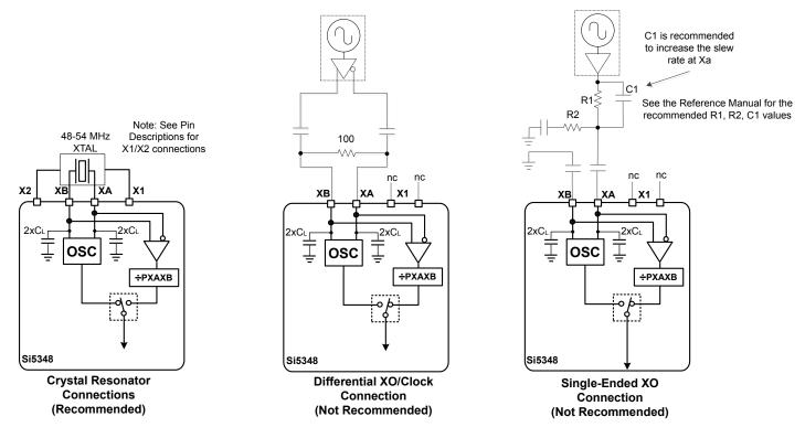
Figure 4.4. Crystal Resonator Connections
