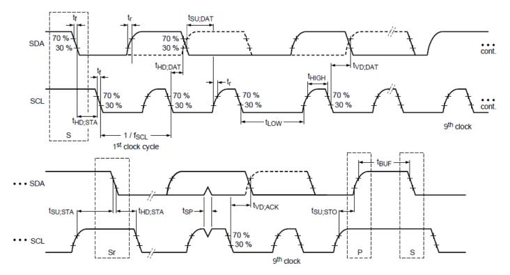
Figure 6.1. I<sup>2</sup>C Serial Port Timing Standard and Fast Modes
