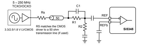
Use R1 and R2 if necessary to keep the signal at REF < 3.6 Vpp\_se. See Reference Manual for details.
