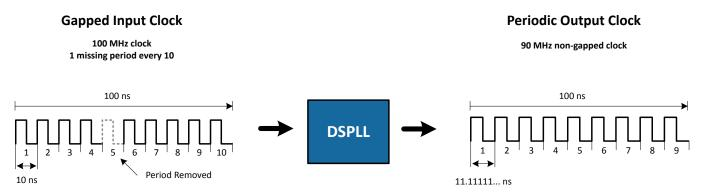
Figure 4.9. Generating an Averaged Clock Output Frequency from a Gapped Clock Input
