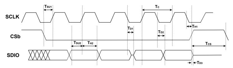
Figure 6.3. 3-Wire SPI Serial Interface Timing
