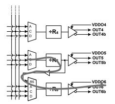
Figure 4.16. Generating a 1 Hz Output using the Si5348
