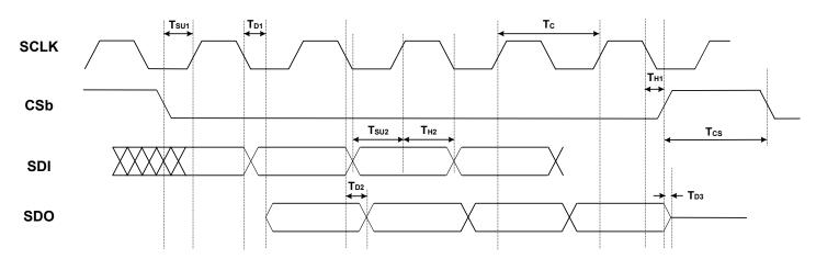
Figure 6.2. 4-Wire SPI Serial Interface Timing
