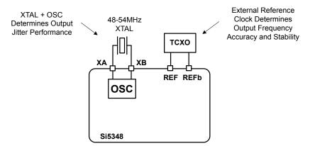
Figure 4.3. External Reference Connections
