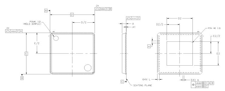
Figure 11.1. Si5348 9x9 mm 64-Pin Quad Flat No-Lead (QFN)
