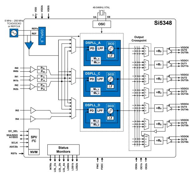
Figure 8.1. Si5348-E Detailed Block Diagram
