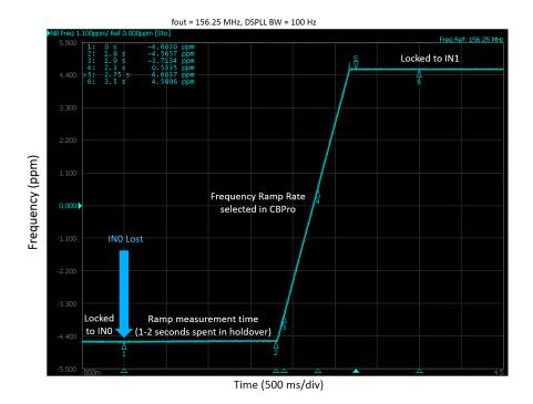
Figure 4.7. Output Frequency Transient-Ramped Switching between Two 8 kHz Inputs (±4.6 ppm Offset)
