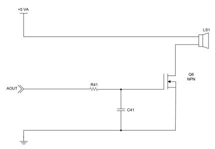
Figure 18. AOUT PWM Circuit for Call Progress
