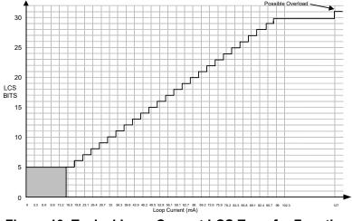
Figure 19. Typical Loop Current LCS Transfer Function
