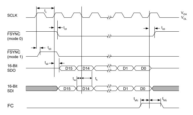
Figure 3. Serial Interface Timing Diagram (DCE = 0)
