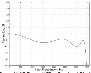
Figure 14. IIR Transmit Filter Passband Ripple
