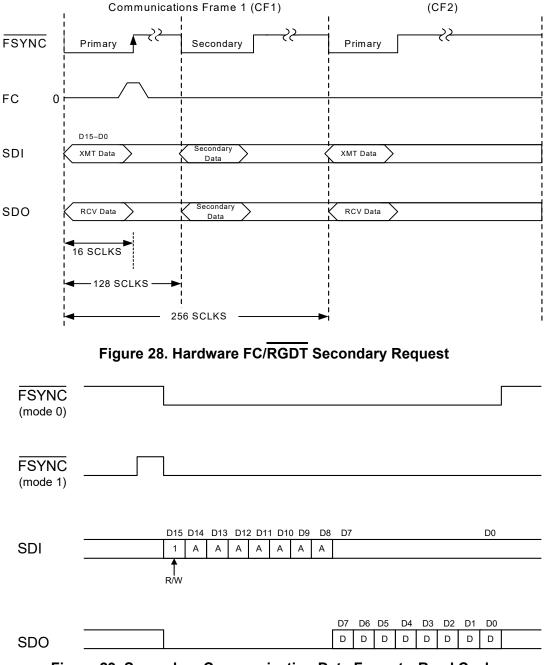
Figure 29. Secondary Communication Data Format—Read Cycle
