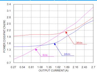
Power dissipation vs. load current at 25°C.
