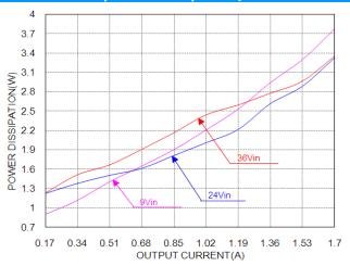
Power dissipation vs. load current at 25°C..
