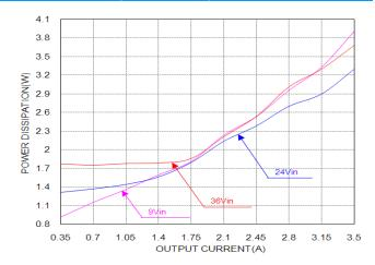
Power dissipation vs. load current at 25°C.
