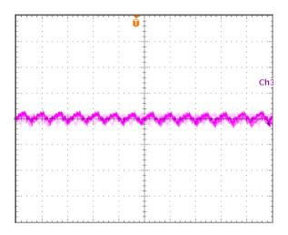
Input reflected ripple current, is, through a  $12\mu H$  source inductor at nominal input voltage and rated load current (25 mA/div, 4us/div)
