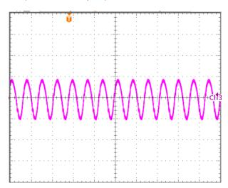
Input Terminal Ripple Current, ic, at full rated output current and nominal input voltage with 12µH source impedance and 100µF electrolytic capacitor (250 mA/div, 4us/div).
