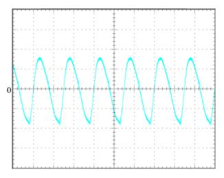
Output voltage ripple at nominal input voltage and max load current (20mV/div, 2us/div)
