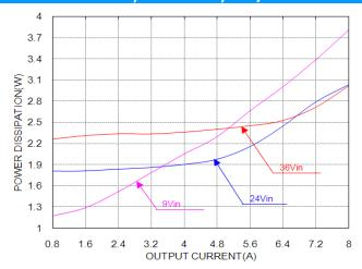
Power dissipation vs. load current at 25°C.
