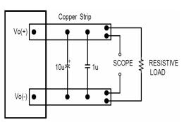
Output voltage ripple test setup.
