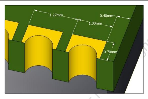
Figure 8. Typical pad dimensions
