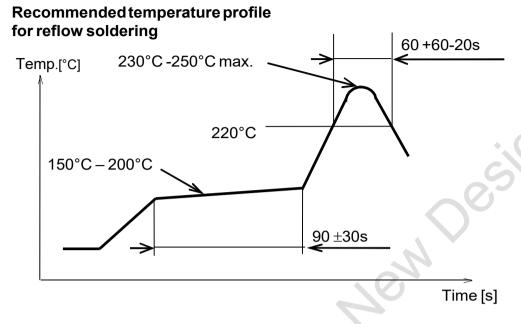
Figure 9. Recommended Reflow Profile
