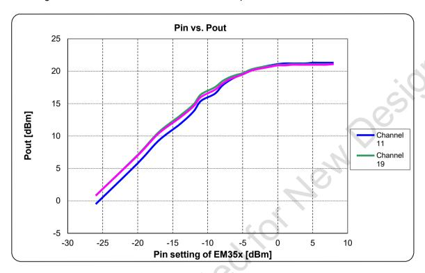
Figure 3. Output Power vs. Power Setting
