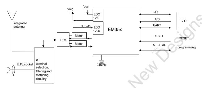
Figure 2. Hardware Diagram
