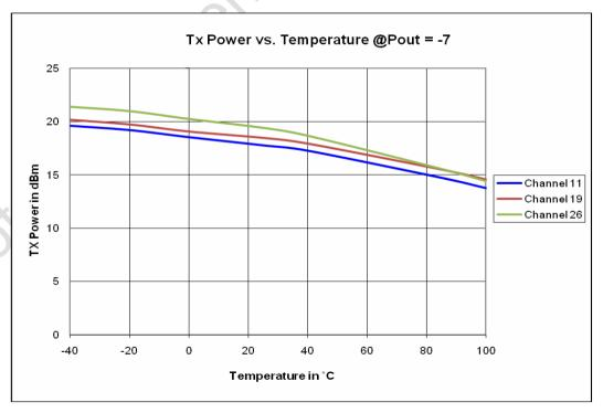
Figure 6. TX Power vs. Temperature
