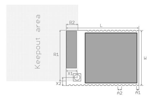
Figure 7. ETRX3 Physical Dimensions
