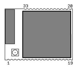
Figure 1. ETRX3 series Module Pinout (top view)
