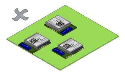
Figure 13. How to not place the Module
