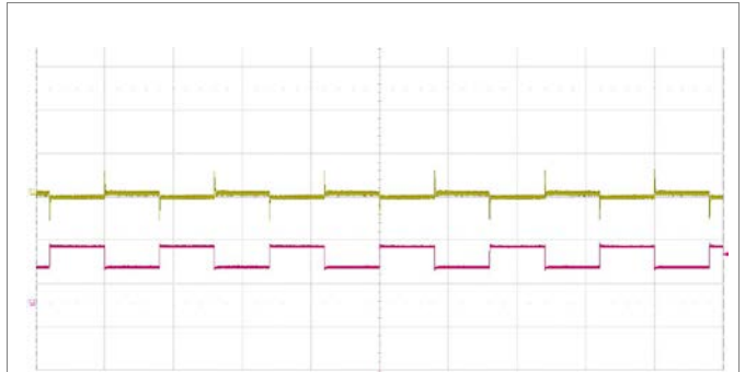
Output voltage response to load current step-change (7.25-10.87-7.25 A) at: T_{P1} = +25^\circ\text{C} , V_i = 110\text{ V} . Top trace: output voltage (500 mV/div.). Bottom trace: load current (5 A/div.). Time scale: (2 ms/div.).
