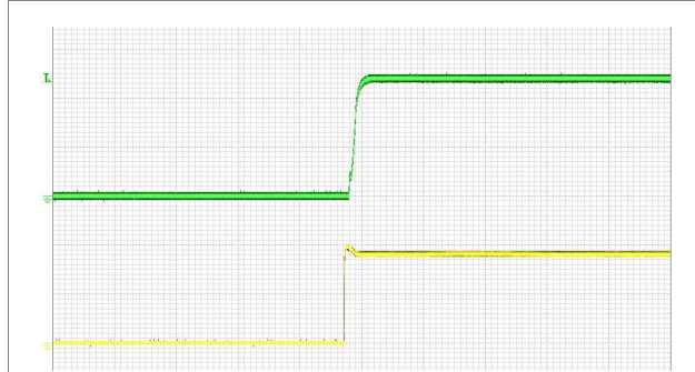
Start-up enabled by connecting V_i at: T_{P1} = +25^{\circ}\text{C} , V_i = 9\text{ V} , I_o = 1.67\text{ A} resistive load. Top trace: output voltage (10 V/div.), Bottom trace: input voltage (5 V/div.). Time scale: (50 ms/div.).
