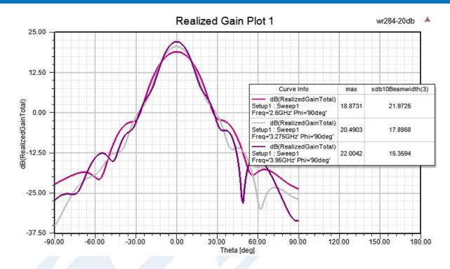
WR-284 Standard Gain Horn with 20 dBi gain, N Female connector from Pasternack Enterprises has same day shipment for domestic and International orders. Our RF, microwave and millimeter wave products maintain a 99.4% availability and are part of the broadest selection in the industry.
