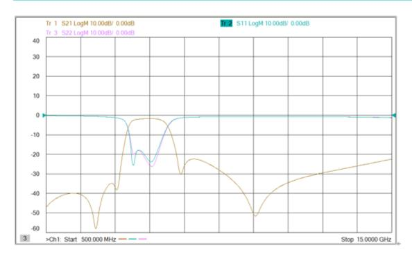
Measured on Agilent E5071C Network Analyzer
