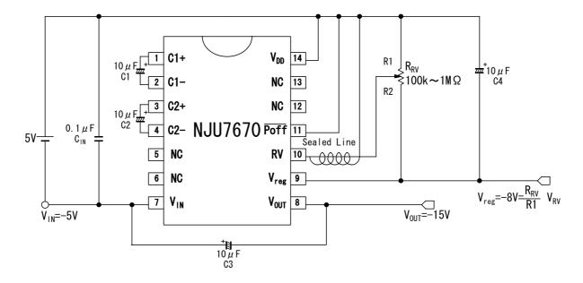
The IC may have a possibility not to operate properly with unstable supply voltage due to large transient current when the capacitor is charged or discharged.
