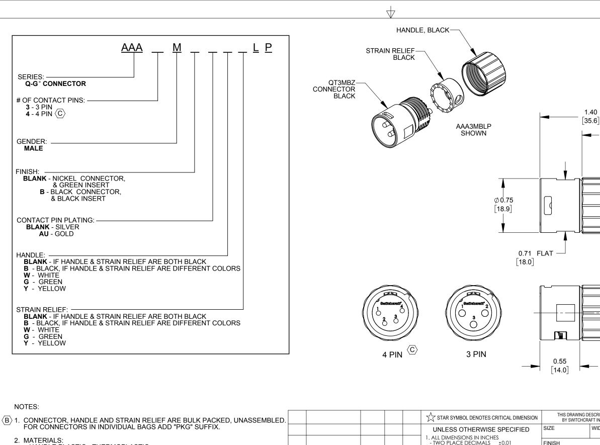
MATERIALS: HANDLE PLASTIC - THERMOPLASTIC STRAIN RELIEF - THERMOPLASTIC HOUSING - ZINC ALLOY, NICKEL PLATED OR BLACK INSULATOR - THERMOPLASTIC, GREEN OR BLACK GROUND TERMINAL - SPECIAL COPPER ALLOY CONTACT PINS - COPPER ALLOY, SILVER PLATED OR GOLD PLATED
