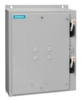
Duplex starter w/ alternator, Size 0, Three phase full voltage, Solid-state overload relay, OLR amp range 3-12A, 110V 50Hz / 120V 60Hz coil, Combination type, Two 10A circuit breakers, Enclosure NEMA type 12, Dust/drip proof for indoors
