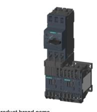
Load feeder fuseless, Reversing duty 400 V AC, Size S00 0.45...0.63 A 230 V AC Spring-type terminal for installation on standard mounting rail (also fulfills type of coordination 1) Type of coordination 2, Iq = 150 kA 1 NC (contactor)
