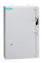
Non-reversing motor starter, Size 3, Three phase full voltage, Solid-state overload relay, OLR amp range 25-100A, Combination type, 125A circuit breaker, Encl NEMA type 4X 316 S-Steel, Water/dust tight noncorrosive, Standard width enclosure
