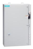
Non-reversing motor starter, Size 3, Three phase full voltage, Solid-state overload relay, OLR amp range 25-100A, 208VAC 60Hz coil, Combination type, 100A non-fusible disconnect, Enclosure NEMA type 4/12, Water/dust tight for outdoors, Standard width enclosure
