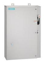
Non-reversing motor starter, Size 2 1/2, Three phase full voltage, Solid-state overload relay, OLR amp range 25-100A, Combination type, 100A fusible disconnect, 100A/600V fuse clip, Encl NEMA type 4X 304 S-Steel, Water/dust tight noncorrosive, Extra-wide enclosure
