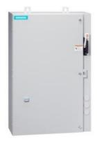
Non-reversing motor starter, Size 1, Three phase full voltage, Solid-state overload relay, OLR amp range 10-40A, 110V 50Hz / 120V 60Hz coil, Combination type, 60A non-fusible disconnect, Encl NEMA type 4X 304 S-Steel, Water/dust tight noncorrosive, Extra-wide enclosure
