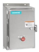
Non-reversing motor starter, Size 2 1/2, Three phase full voltage, Amb. compensate bimetal OLR, Contactor amp rating 60A, 208VAC 60Hz coil, Non-combination type, Encl. type 4X 304 S. Steel, Water/dust tight noncorrosive
