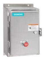
Non-reversing motor starter, Size 2, Three phase full voltage, Solid-state overload relay, OLR amp range 13-52A, 24VAC 50-60Hz coil, Non-combination type, Encl. type 4X 304 S. Steel, Water/dust tight noncorrosive, Standard width enclosure
