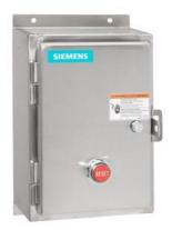
Non-reversing motor starter, Size 2, Three phase full voltage, Solid-state overload relay, OLR amp range 13-52A, Non-combination type, Encl. type 4X 304 S. Steel, Water/dust tight noncorrosive, Standard width enclosure
