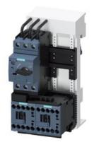
Load feeder fuseless, Reversing duty 400 V AC, Size S00 1.10...1.60 A 230 V AC screw terminal for 60 mm busbar systems (also fulfills type of coordination 1) Type of coordination 2, Iq = 150 kA 1 NC (contactor)
