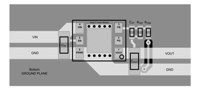
The picture above shows a possible layout for the 171010501 Magl<sup>3</sup>C MicroModule. Nevertheless, some recommendations should be followed when designing the layout:
