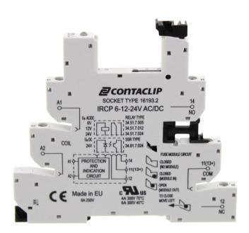
Interface-Relay-Compact (IRC) socket base IRC with screw connection, Mounting type: Mounting rail TS 35, 1 CO contact, Input voltage: 6, 12 or 24 VAC/DC
