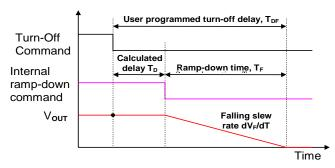
As it can be seen from the figure, the internally calculated delay  $T_{\text{D}}$  is determined by the equation below.
