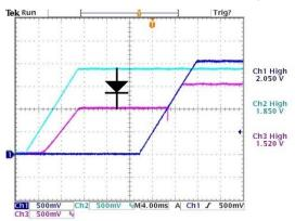
Figure 29 was captured with an actual system where a diode was added to pre-bias a 1.5V bus from a 1.85V bus in order to simulate the effect of current leakage through protection circuits of unpowered logic connected to powered logic outputs (a common source of pre-bias in power systems).
