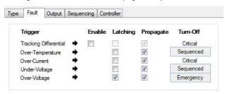
If the non-latching protection is selected, a dPOL will attempt to restart every 130ms until the condition that triggered the protection is removed. When restarting, the output voltages follow tracking and sequencing settings.
