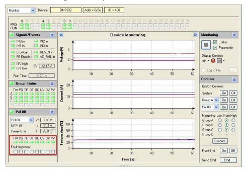
Figure 56. Fault Injection Controls In Monitor Window
