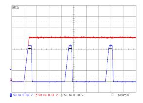
Since both Vo1 and Vo2 have the same delay and slew rate settings they will continue to turn off and on synchronously every 130ms as shown in Figure 43 until the condition causing the undervoltage is removed.
