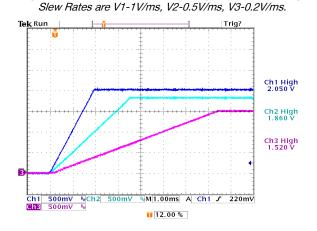
Figure 26. Turn-On with Different Rising Slew Rates. Rising
