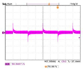
Figure 53. Transient Response with Regulation set to 0.74 mV/A
