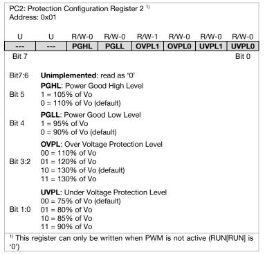
Note that the overvoltage and undervoltage protection thresholds and Power Good limits are defined as percentages of the output voltage. Therefore, the absolute levels of the thresholds change when the output voltage setpoint is changed either by output voltage adjustment or by margining.
