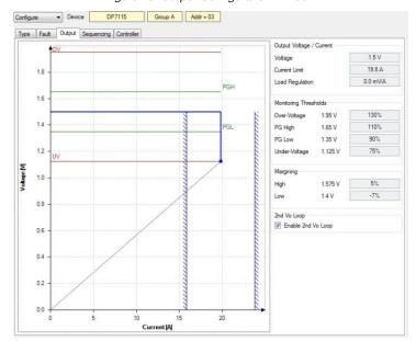
Figure 15. Output Configuration Window
