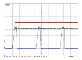
Figure 41 shows a scope capture an actual system when undervoltage error detection is set to not propagate.
