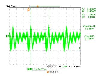
Figure 48. Input Voltage Noise with Interleave
