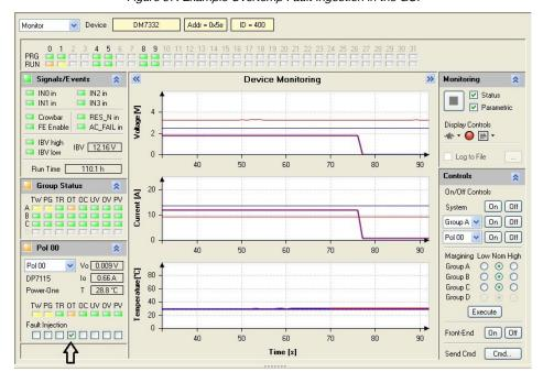
Figure 57. Example Overtemp Fault Ingection in the GUI
