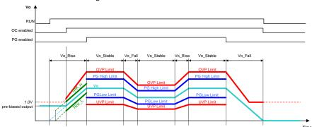
Figure 34. Protection Enable Conditions
