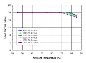
Figure 3. Available output current vs. ambient air temperature and airflow rates for converter DP7120G mounted horizontally with air flowing from input to output, MOSFET temperature ≤ 120 °C, Vin = 12 V, Vout = 5 V, and Fsw= 500KHz
