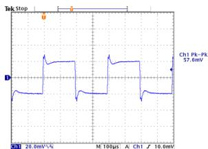
As the Load Regulation parameter is increased, step offsets in output voltage begin to appear, as shown in Figure 19 with non-zero Regulation.
