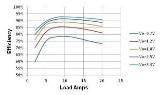
Figure 7 Efficiency vs Vout at Vin=12V, Load=20A
