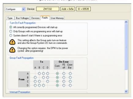
Note that the turn-off type of the fault as it propagates through the DPM will remain unchanged. Propagation options for dPOLs can be read or set in the dPOL PC3 register shown in Figure 38.
