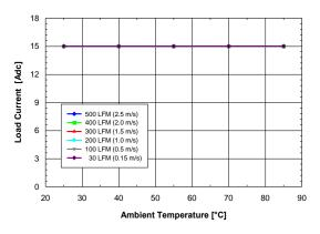
Figure 4. Available output current vs. ambient air temperature and airflow rates for converter DP7120G mounted horizontally with air flowing from input to output, MOSFET temperature ≤ 120 °C, Vin = 12 V, Vout = 5 V, and Fsw= 1MHz
