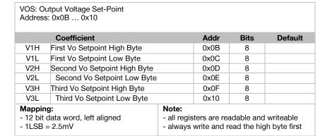
Figure 16. Output Voltage Setpoint Register VOS
