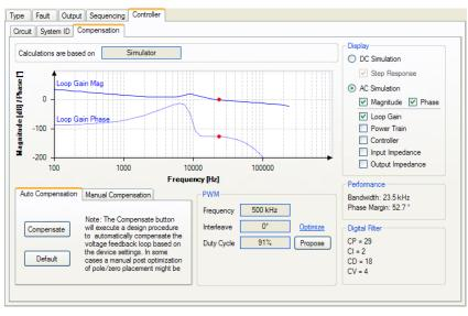
Figure 45. PWM Controller Window
