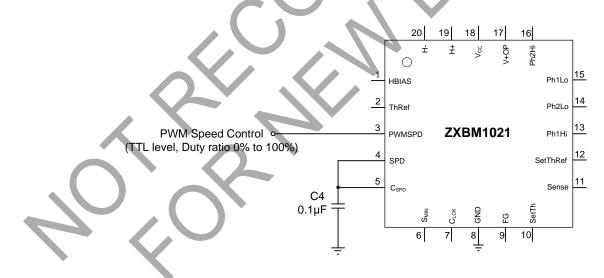
When using PWMSPD speed input, the SPD pin should be connected to C<sub>SPD</sub> with a 0.1µF capacitor connected to ground. PWMSPD can be driven from a microcontroller with either 0-5V or 0-3.3V logic levels signal. The recommended frequency of the input PWM control signal is 25kHz.
