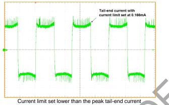
(Tail-end current = 145mA typ, Current limit set at 0.166mA)
