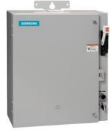
Pump control panel, Size 1 3/4, Three phase full voltage, Solid-state overload relay, OLR amp range 10-40A, 380-440/440-480V 50/60Hz coil, Standard type contactor, 40A circuit breaker, HOA Sel Sw. <(>&<)> Start P.B., Enclosure NEMA type 3/3R, Weather proof outdoor use
