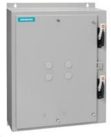
Duplex starter w/o alternator Size 3.5 Three phase full voltage Solid-state overload relay OLR amp range 50-200A 240VAC 50Hz / 277VAC 60Hz Coil Combination type Two 200A disconnect switches Encl NEMA type 4 painted steel Water/dust tight weather proof
