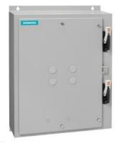
Duplex starter w/o alternator Size 3.5 Three phase full voltage Solid-state overload relay OLR amp range 50-200A Combination type Two 200A disconnect switches Encl NEMA type 4 painted steel Water/dust tight weather proof
