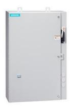
Non-reversing motor starter, Size 2 1/2, Three phase full voltage, Solidstate overload relay, OLR amp range 25-100A, Combination type, 100A circuit breaker, Encl NEMA type 4X 316 S-Steel, Water/dust tight noncorrosive, Standard width enclosure
