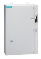
Non-reversing motor starter, Size 1 3/4, Three phase full voltage, Solid-state overload relay, OLR amp range 10-40A, 24VDC coil, Combination type, 60A fusible disconnect, 60A/250V fuse clip, Enclosure NEMA type 4/12, Water/dust tight for outdoors, Extra-wide enclosure
