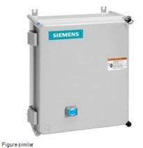
Non-reversing motor starter, Size 3 1/2, Three phase full voltage, Solid-state overload relay, OLR amp range 50-200A, Non-combination type, Enclosure type 4X fiberglass, Water/dust tight noncorrosive, Standard width enclosure
