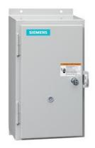
Non-reversing motor starter, Size 2 1/2, Three phase full voltage, Amb. compensate bimetal OLR, Contactor amp rating 60A, Non-combination type, Enclosure type 12, Dust/drip proof for indoors
