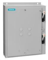
Duplex starter w/o alternator, Size 2 1/2, Three phase full voltage, Solidstate overload relay, OLR amp range 25-100A, 24VAC 50-60Hz coil, Combination type, Two 100A circuit breakers, Encl NEMA type 4X 304 S-Steel, Water/dust tight noncorrosive
