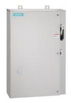
Non-reversing motor starter, Size 4, Three phase full voltage, Solid-state overload relay, OLR amp range 50-200A, 110V 50Hz / 120V 60Hz coil, Combination type, 150A circuit breaker, Encl NEMA type 4X 316 S-Steel, Water/dust tight noncorrosive, Standard width enclosure
