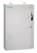
Non-reversing motor starter, Size 2 1/2, Three phase full voltage, Solid-state overload relay, OLR amp range 25-100A, Combination type, 60A fusible disconnect, 60A/600V fuse clip, Encl NEMA type 4X 304 S-Steel, Water/dust tight noncorrosive, Extra-wide enclosure
