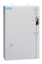
Non-reversing motor starter, Size 2 1/2, Three phase full voltage, Solidstate overload relay, OLR amp range 25-100A, 24VDC coil, Combination type, 100A fusible disconnect, 100A/600V fuse clip, Enclosure NEMA type 4/12, Water/dust tight for outdoors, Extra-wide enclosure
