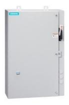
Non-reversing motor starter, Size 0, Three phase full voltage, Solid-state overload relay, OLR amp range 0.25-1A, 24VDC coil, Combination type, 30A fusible disconnect, 30A/250V fuse clip, Enclosure NEMA type 4/12, Water/dust tight for outdoors, Extra-wide enclosure
