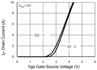
**Figure 7 Transfer Characteristics**
