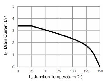
**Figure 4 Drain Current**
