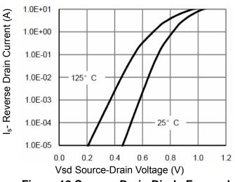
Figure 12 Source- Drain Diode Forward
