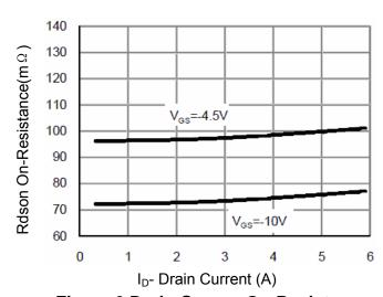
Figure 6 Drain-Source On-Resistance
