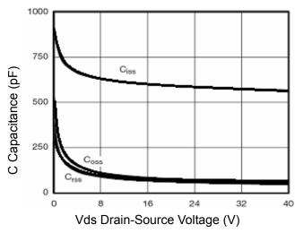
Figure 10 Capacitance vs Vds
