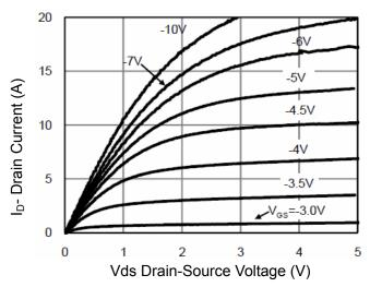
**Figure 5 Output Characteristics**
