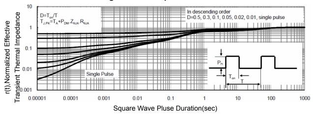
**Figure 14 Normalized Maximum Transient Thermal Impedance**
