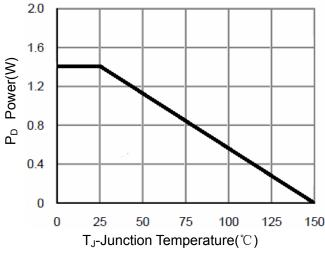
**Figure 3 Power Dissipation**
