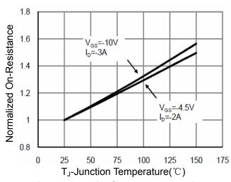
Figure 8 Drain-Source On-Resistance
